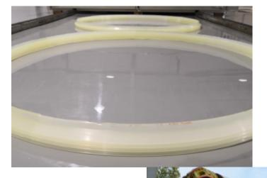
In addition to machined seals, UTEC Sealing Solutions has also improved the production process for seals for Tunnel Boring Machines (TBM). At our facilities in Suzhou, we can produce virtually any seal size for TBMs out of Polyurethane.
