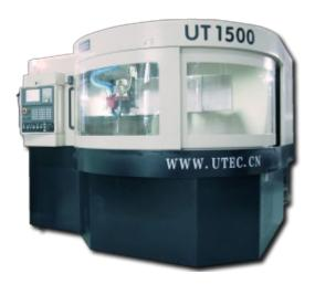
All UTEC seal machining systems come fully equipped with a 12-station hydraulic tool turret, chip cutter, powerful suction unit, a set of tools and high-quality aluminum chuck jaws.
